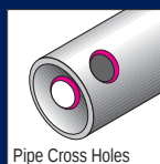
Pipe Cross Holes
